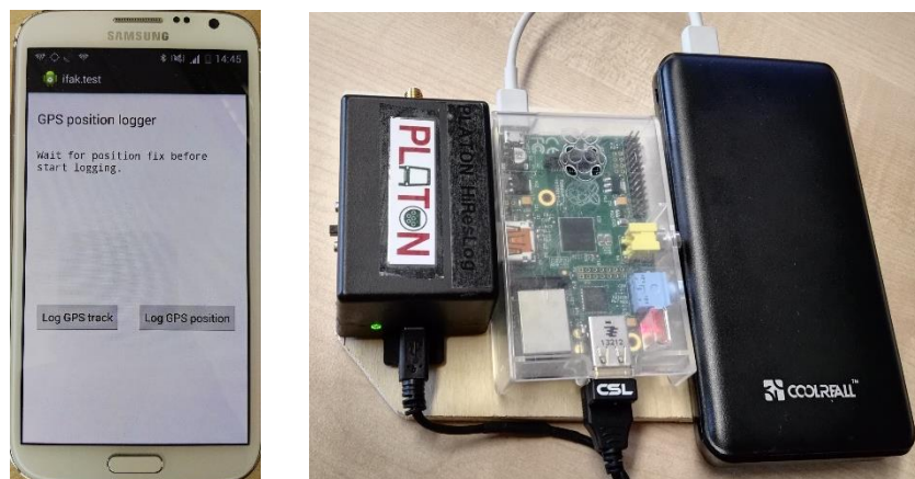
Figure 13 CollectApp implementation in smartphone (left) and Raspberry Pi Logger device (right).
